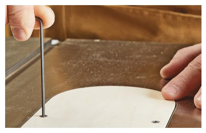
Once the insert is set in place, use an Allen wrench to adjust each set screw until the insert is flush with the saw table.
